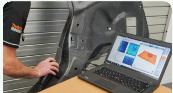
Figure 6. A two-dimensional array 'ultrasonic camera' used by Thatcham Research to inspect a complex composite component
